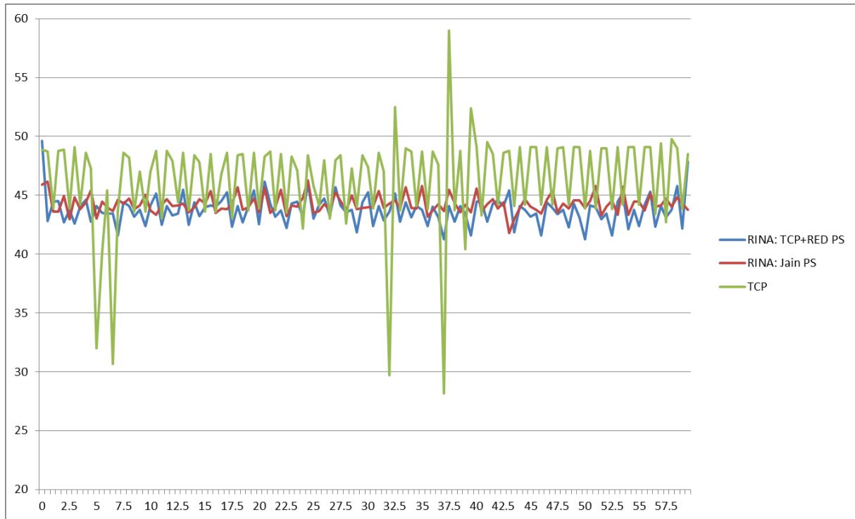
Figure 12. Two hosts experiment, single flow: Throughput (Mbps) vs. Experiment time (s)
